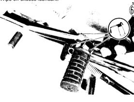
•Force grease into the fitting until it comes out at both sides of the swing arm, and wipe off any excess.
