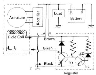
Fig. 562 shows a basic circuit of the regulator that is referred to in the following explanation.
