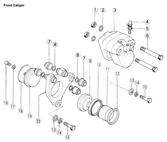
Nut Spacer Caliper Bleed Valve Cap Bleed Valve
