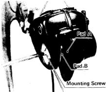
•After pad B is removed, slide the caliper body to the right side of the motorcycle and remove pad A. **NOTE:** If it is difficult to take out pad A, squeeze the brake lever several times until the caliper piston pushes it out.
