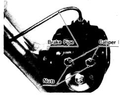
•Unscrew the brake pipe from where it connects to the
