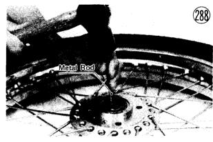
•Insert a metal rod into the hub from the speedometer
