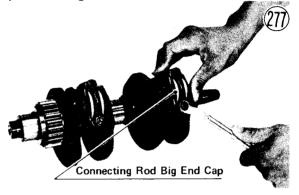
•Remove the rod bearing insert halves from the connecting rod big end and the big end cap.
