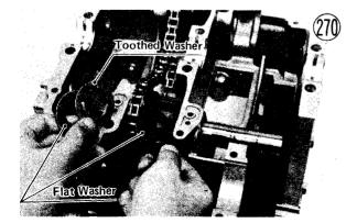
•Apply oil to each shaft, and insert them keeping the chain on the sprockets. Match the shaft hole with the hole in the balancer weight. The rear balancer weight shaft has the engine oil pump driver gear on its left end. Be sure that all washers are in place and that the sprockets are on the left side of the weights.
