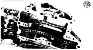
•Use a new lock washer, apply a non-permanent locking agent to the threads of the mounting bolts. Check to see that the balancer chain timing is correct, then bend the sides of the washer over against the balancer chain tensioner bolts (2). The tightening torque of the mounting bolts is 0.9 ~ 1.1 kg-m (78 ~ 95 in-lbs).
