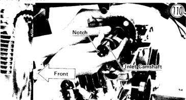
•Remove the camshaft cap bolts (16), and take off the camshaft caps (8).
