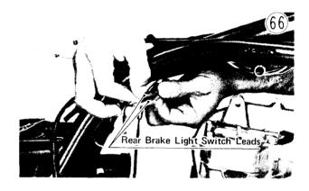
Remove the rear brake light switch spring
