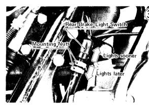
Caution To avoid damaging the electrical connections inside the switch, be sure that the switch body does not turn during adjustment.
