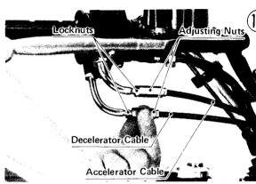
•Turn out the decelerator throttle cableadjusting nut 3 turns. There must still be play in the throttle grip; if there is not, loosen the locknut at the lower end of the decelerator cable, turn in the adjuster to small create а amount of play, and retighten the locknut. worn.
